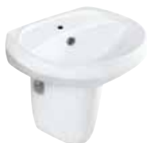
SLS-WHT-6801 Half pedestal basin Wall Hung Basin with Fixing Accessories Size: 575x465x200 mm Rs. 4,350 SLS-WHT-6305 Half pedestal with Fixing Accessories for SLS-WHT-6801 Rs. 1,700 Set (MRP) Rs. 6,050
